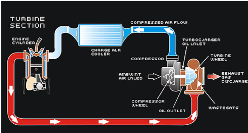
The amount of density regained depends on the ambient temperature of the air (in air-to-air units), the efficiency of the compressor (max boost, wheel efficiency etc.) and the cooling capacity of the intercooler.
